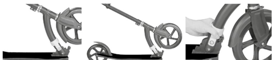
Lift the plastic rim of the disassembling mechanism of the vehicle upwards. Then lift the steering column until it reaches a vertical position and you hear a click indicating its correct position. The disassembling mechanism will automatically lock.
