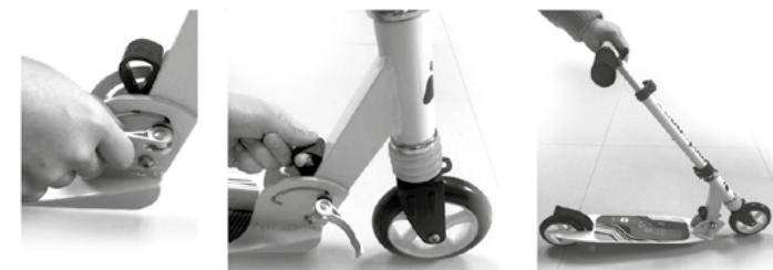
Unlock the lock of a mechanism for disassembling the product by lifting the lever, then lift the plastic element of the disassembling mechanism of the vehicle upwards to release the disassembling lock. Lift the steering column to the vertical position until you hear a click indicating that the steering wheel is in the correct position. Clutch the lock of the disassembling mechanism. If after locking the steering column you can still move it, tighten the nut on the opposite side than the lever.
